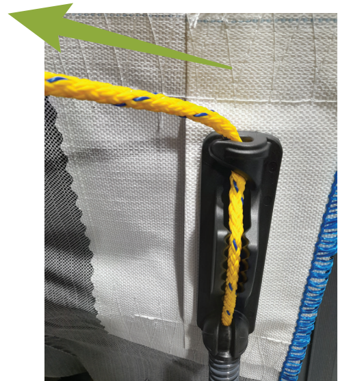
Figure 11: Locking the rope and the direction of pulling
