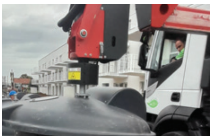
Figure 23: Connecting the vehicle lifting mechanism to the lifting mechanism of the container
