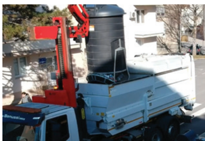
Figure 25: Lifting and emptying the insert
