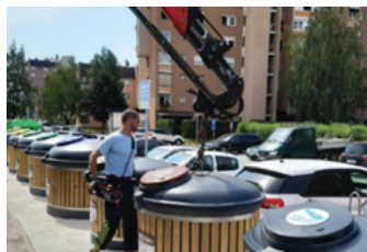
Figure 16: Fasten the hook of the lifting mechanism to the hook
